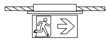
option montage encastré en utilisant le kit option with recessed mount kit applied
